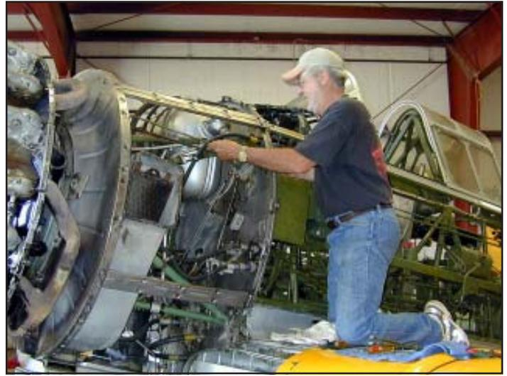
Col Dan Duewall installs new fabric boots on the control rods of Col Coombes' SNJ. Besides being a talented pilot, Dan is also an aircraft mechanic (A&P) and has donated a great deal of his time and talent to keep the Wing aircraft flying.
