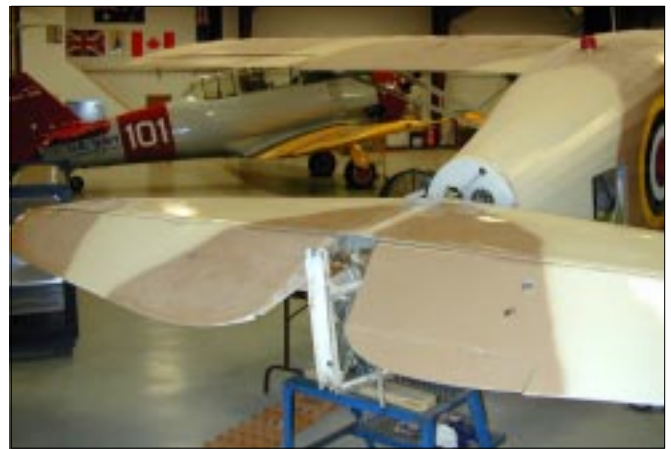
The Bad News — the Tar-Baby's tail is missing while repairs to the woodwork and fabric are being done. Note the larger than normal holes from the fabric test!
