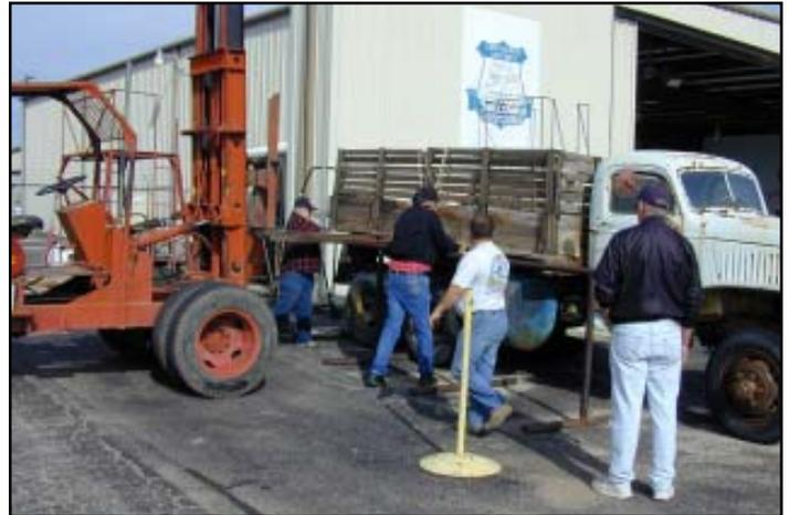
After all bolts and attachments were removed, it came time to lift the bed onto the support rails, after which the plan was to drive the truck out from under the bed.
