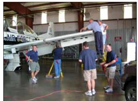
The inspection of the T-28A showed the airframe was in good condition for its age but the engine was making metal and in need of an overhaul. Thanks to T-28 guru Bill Muszala we knew the exact condition of the plane before making our request for assignment. More at the meeting.
