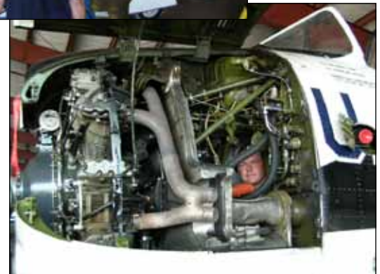
Here I am the hydraulic pumper for the gear swing tests as we didn't have the correct fittings for the mule.
