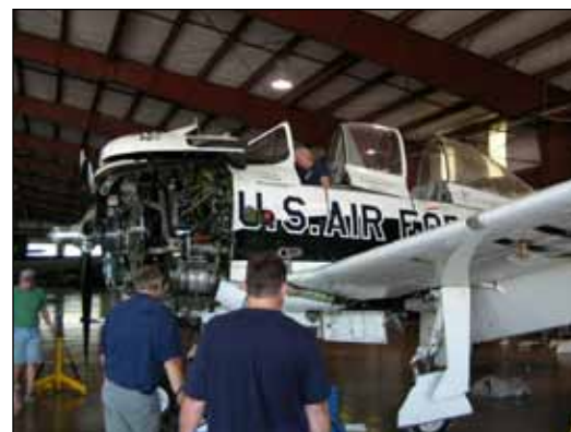
The inspection of the T-28A showed the airframe was in good condition for its age but the engine was making metal and in need of an overhaul. Thanks to T-28 guru Bill Muszala we knew the exact condition of the plane before making our request for assignment. More at the meeting.
