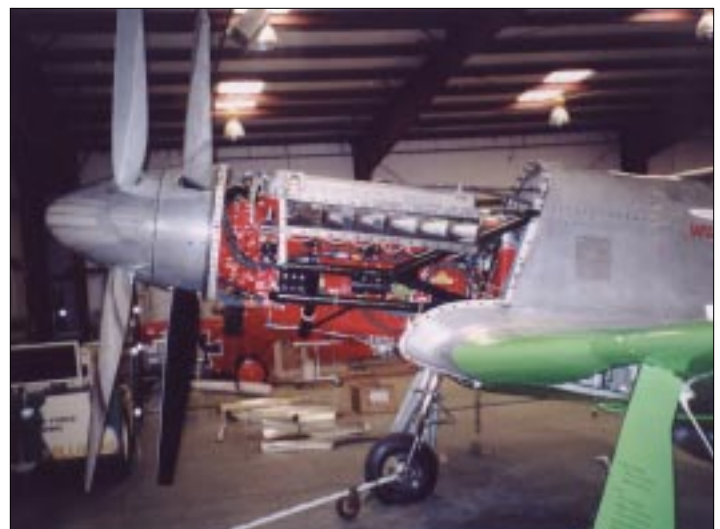
The Rolls-Royce Griffon engine and counter-rotating props are a tight fit in the nose of Precious Metal .
