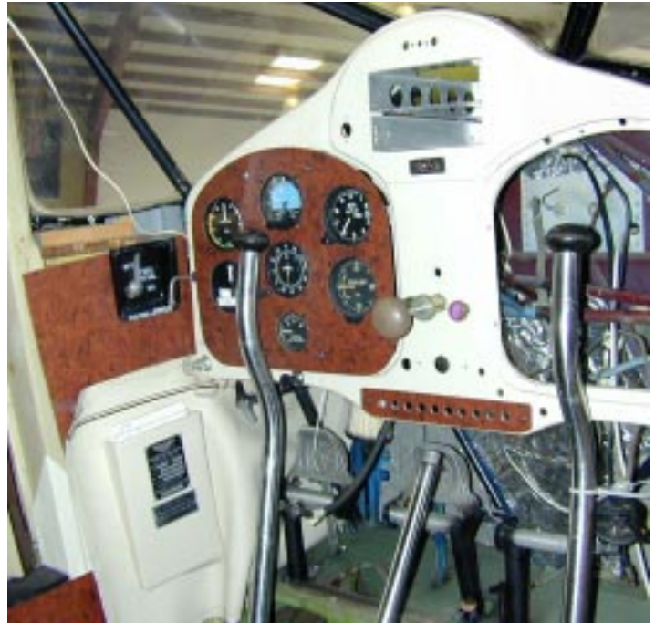
The left side of the new instrument panel of the UC-61/Argus being test fitted. Things are going back together.
